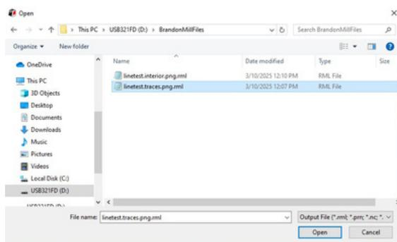
This should open the File Explorer. Navigate to the location of the RML file and select it, then click the 'Open' Button. Ensure that you select the correct file for the end mill that is loaded in the machine!
