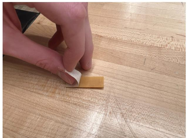
Remove the double sided tape from the back of the FR1 and board.
