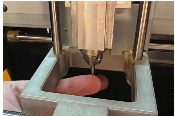
Remove an end mill by loosening the collet using the hex key on the right side of the machine. Careful, it will drop if not held! Load an end mill by pushing it up into the collet and tightening using the hex key.
