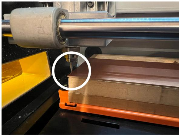
Bring the tip of the end mill close to **but not touching** the bottom left corner of the FR1. Then, hit the **X/Y** button in the Setting Origin section of VPanel. Confirm the change by selecting 'yes' when asked to continue. The X and Y position in the Positional Information section of VPanel should both change to 0.00 mm
