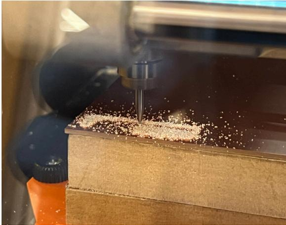
It is normal for there to be dust while milling. Too much dust indicates the end mill may be too deep (too much pressure while setting Z origin) and too little dust indicates the end mill may be too shallow (too little pressure while setting the Z origin)
