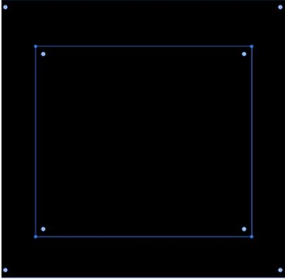
Start by opening the *Edge\_Cuts.svg* file in Adobe Illustrator. It should consist of a black shape with a faint white outline of the edge designed in KiCad. The program to generate tool paths requires the edge cut to be defined as a solid white shape surrounded by a thick black border.
