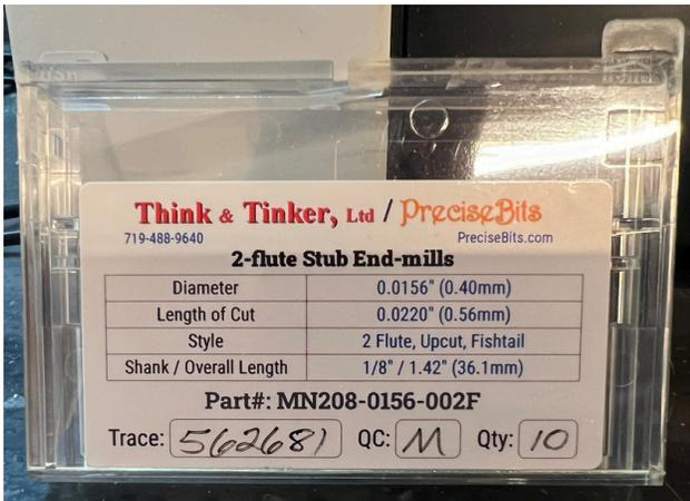
The **0.0156" (0.4mm)** diameter end mills are for milling traces
