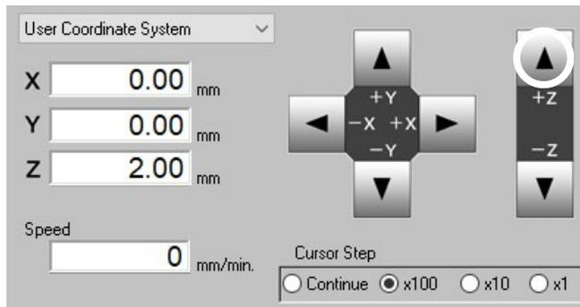
Assuming the Z origin was just set and the end mill is touching the FR1, increase the +Z position by about 2.00 mm. This ensures that the end mill can freely spin when the job begins.
