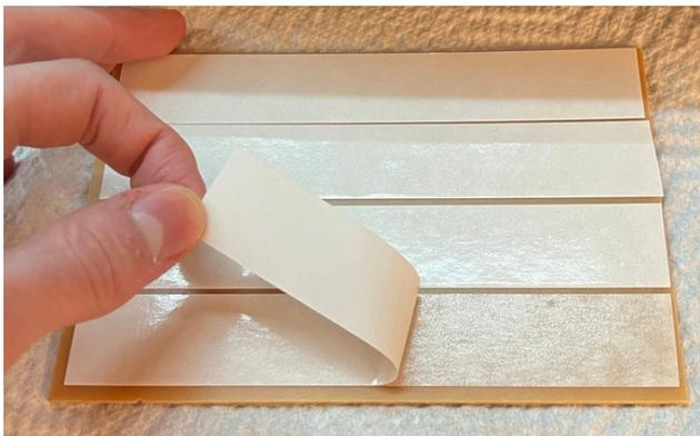
Place double-sided tape to cover the bottom surface of the FR1. Try to avoid air bubbles, overlapping the tape, or any other imperfections that could cause the sheet to lay unevenly when placed in the machine.
