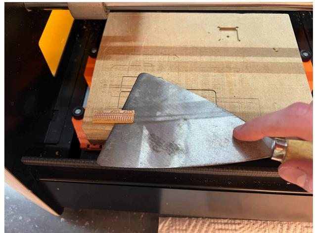
Use a metal scraper to gently lift the FR1 and the milled board from the bed. Try not to bend either as the material can easily crack.
