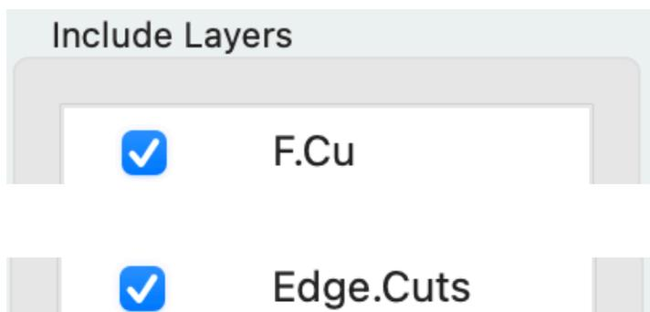
In the **Include Layers** section, select both **F.Cu** and **Edge.Cuts** and ensure that no other layers are selected. This ensures that only these two layers are exported.
