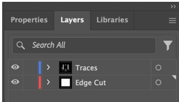
Place the *F\_Cu.svg* and *Edge\_Cuts.svg* onto their own respective layers. An easy way to do this is to select a layer, right click the object to move, then select **Arrange → Send to Current Layer**.
