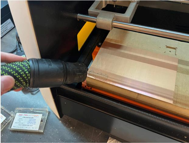
Remove all of the dust from the top of the board with the vacuum. **Try not to make contact with the board as this can damage the delicate traces.** Also vacuum all of the remaining dust from the walls and around the bed of the machine
