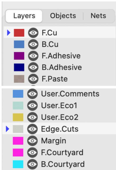
In the KiCad PCB Editor, draw all traces on the **F.Cu** Layer. This stands for “Front Copper.” Draw all shapes that define the edge of the board on the **Edge.Cuts** Layer.
