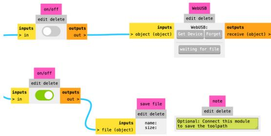
Disable the **on/off** module that connects to the **WebUSB** module and enable the **on/off** module that connects to the **save file** module. The location of these modules is shown below
