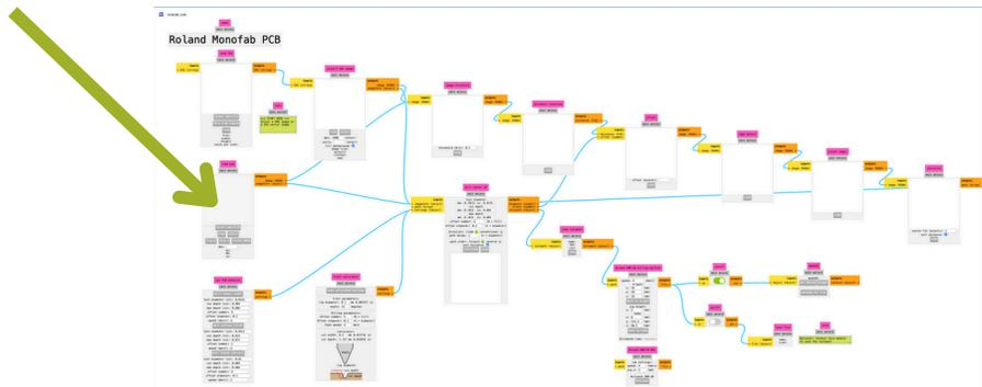
In the **Roland SRM-20 milling machine** module, change **speed** to 10, and **x**, **y**, and **z** to 0. The location of the module is shown below.
