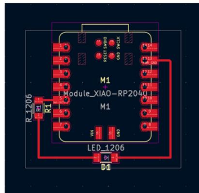
The Shapes on the **Edge.Cuts** should appear as faint outlines and traces on **F.Cu** should be bold and more visible.
