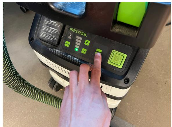
Use the FESTOOL vacuum to remove the dust after each process. Activate the vacuum by powering it on with the power button (left), then enable the suction by lightly pressing the MAN button (right).
